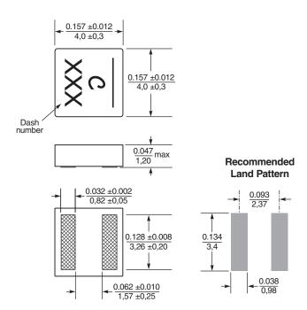
Dimensions are in  $\frac{\text{inches}}{\text{mm}}$
