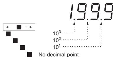
Select the decimal position with the slide switch under the cover on the front panel (signal monitor only).
