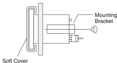
**Note:** Be sure to use the Water-resistant Soft Front Cover and mounting bracket together.
