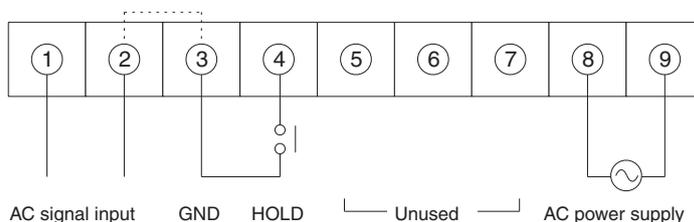
**Note:** Terminals 2 and 3 of the models are not internally insulated. Connect a relay with high contact reliability and insulation (with a minimum load current of 0.3 mA) or a photocoupler with high insulation (with a residual voltage of 1 V max. and a current leakage of 0.1 mA max.) to these terminals for external control.
