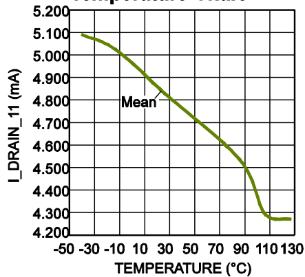
I_DRAIN_11 vs. Temperature Chart
