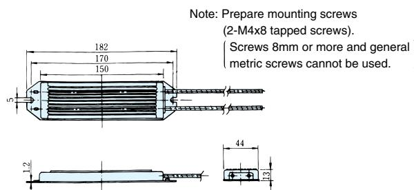
**Braking resistor unit (separately-installed type)**
