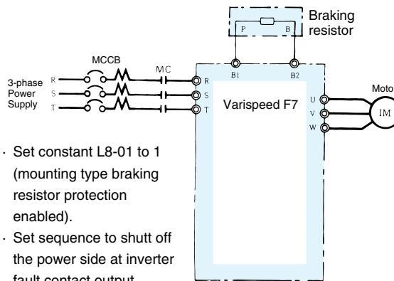
**Connections for braking resistors**
