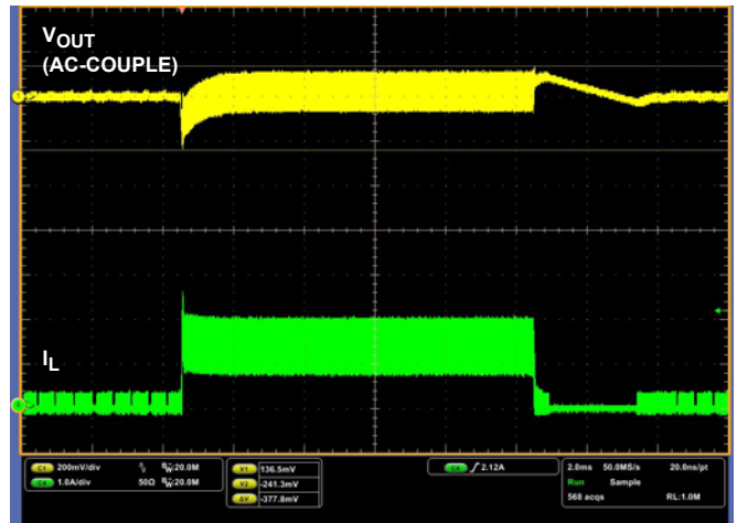
FIGURE 11. LOAD TRANSIENT RESPONSE 0A->1A, VIN = 36V
