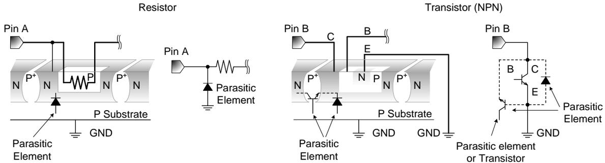
Figure 103. Example of Monolithic IC Structure
