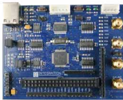
Figure 2. MSC-DKLB2 (Not Included) Testing Platform for controlled Lab Tests (Loadboard)
