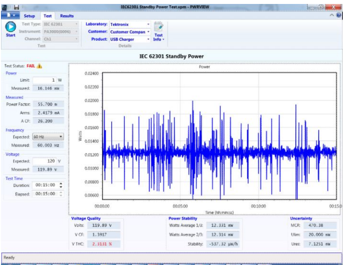
Full compliance IEC 62301 ED 2.0 Standby Power testing with PWRVIEW
