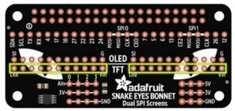
If using TFT or IPS display(s): use the "lower" rows (with the word "TFT" between them).
