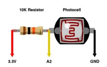
To have the pupils contract or expand in response to light, connect a photocell and 10K resistor in series. The midpoint connects to analog pin **A2**.
