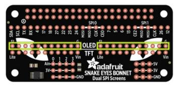
**If using OLED display(s):** use the "upper" rows (with the word "OLED" between them).
