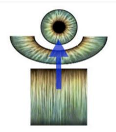
The graphics are stored flat and unrolled, like a map projection. The horizontal (X) axis works like the longitude, or angle around the eye, while the vertical (Y) axis is the latitude.
