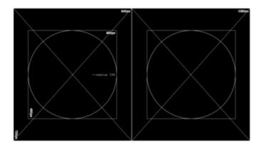
There's a lot of unused blank space around the eyes; this is normal and by design. If developing your own code, this allows you to put debugging or status information in the margins of the HDMI display, but not have it copied to the SPI screens. Also, the eyelids are rendered by dynamically generating 2D meshes, and these need to be a little larger than the eyes to fully block things out. If the eyes were right up against each other, these would overlap.
