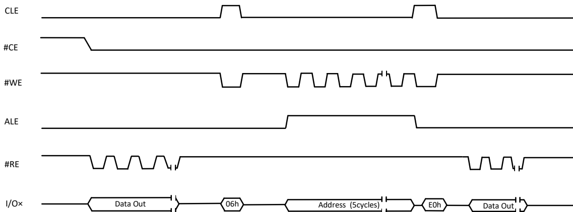
Figure 9-4 Two Plane Random Data Read (06h-E0h) Operation
