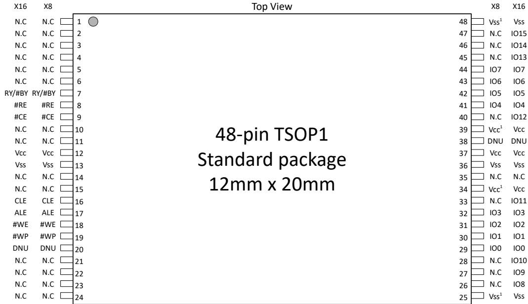
Figure 3-1 Pin Assignment 48-pin TSOP1 (Package code S)
