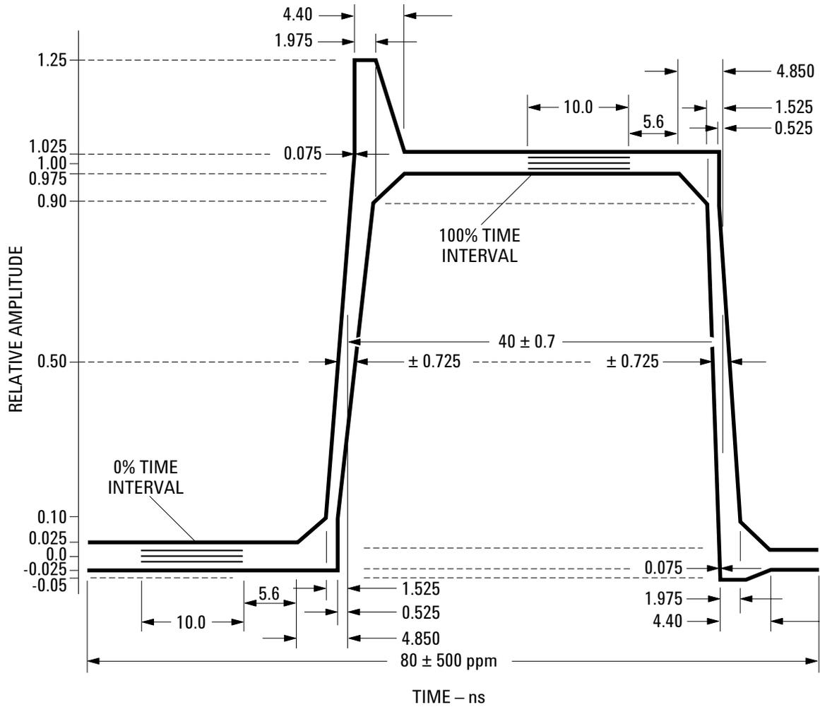
THE AFBR-5103Z OUTPUT OPTICAL PULSE SHAPE SHALL FIT WITHIN THE BOUNDARIES OF THE PULSE ENVELOPE FOR RISE AND FALL TIME MEASUREMENTS.
