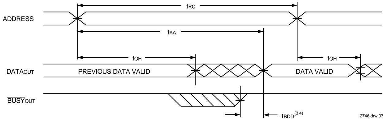
**TIMING WAVEFORM OF READ CYCLE NO. 2, EITHER SIDE<sup>(5)</sup>**
