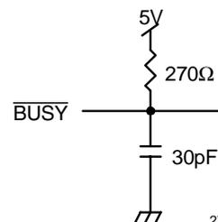
Figure 3.  $\overline{BUSY}$  Output Load
