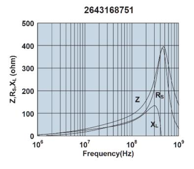
Impedance, reactance, and resistance vs. frequency.
