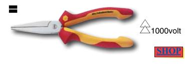
32810 Long Flat Nose Pliers. Insulation According to VDE 0682/part 201, EN/IEC 60900, ASTM F-1505-01, NFPA70E and CSA,  $\stackrel{\frown}{\sim}$  up to 1000 Volt. Individually Tested. DIN ISO 5745 Extra long head. Serrated Jaws are induction hardened. Special C70 tool steel forgings, Chrome finish. Two component Soft Grip handles. Use for Gripping and right-angle bending of wires and sheet metal parts.
