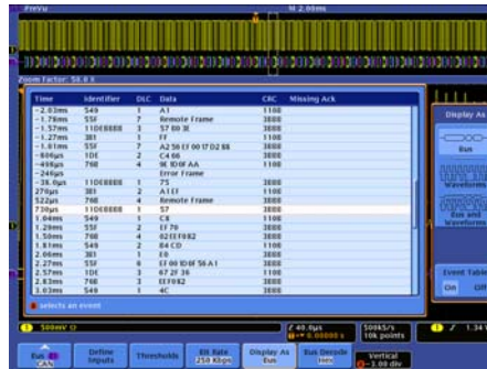
CAN event table display of bus content for easy comparison with software listings.
