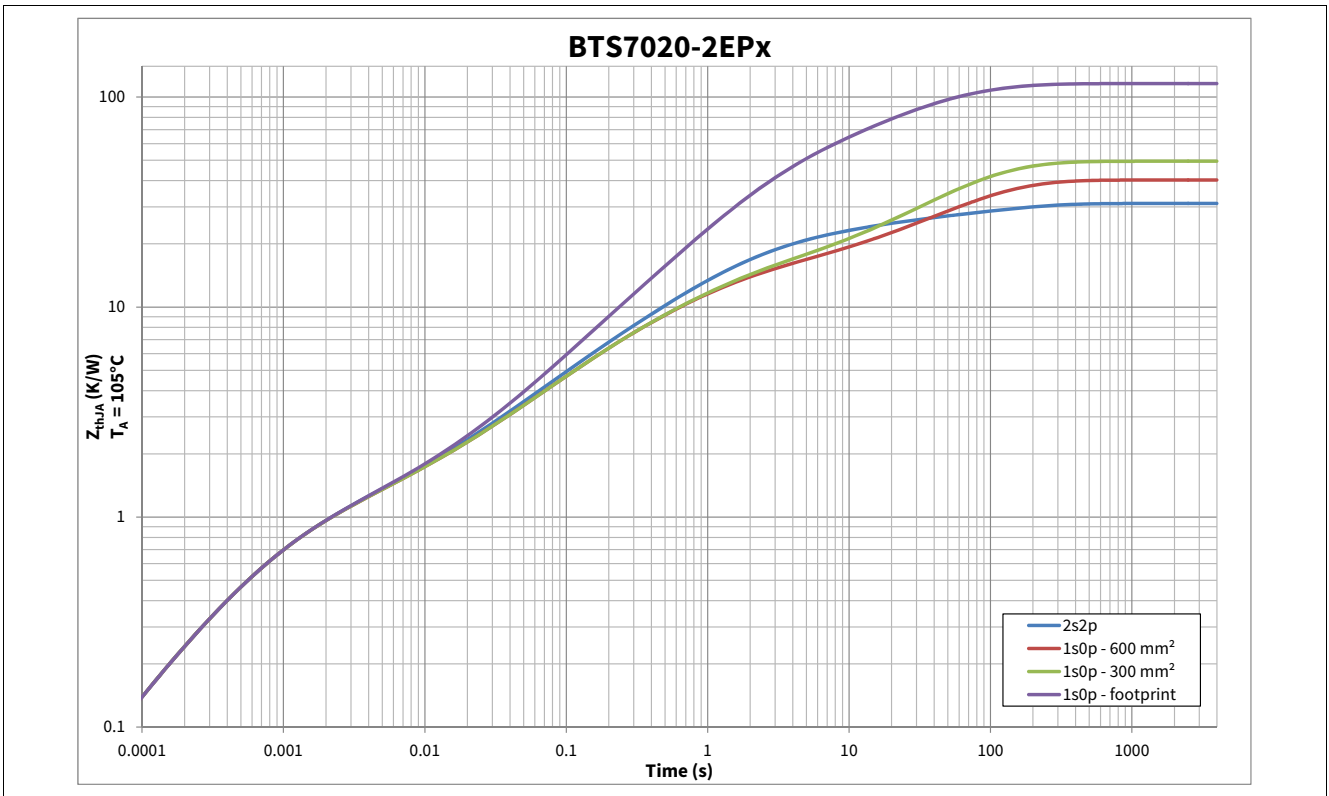
Figure 9 Typical Thermal Impedance. PCB setup according Chapter 4.4.1
