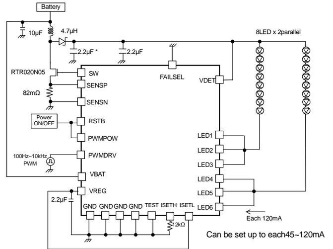
Figure 59. 8 series x 2 parallel, LED current 120mA setting
