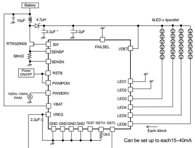
Figure 53. 6 seriesx4 parallel, LED current 40mA setting Current driver PWM application
