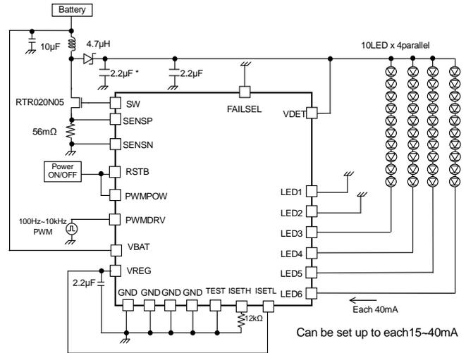
Figure 51. 10 seriesx4 parallel, LED current 40mA setting Current driver PWM application
