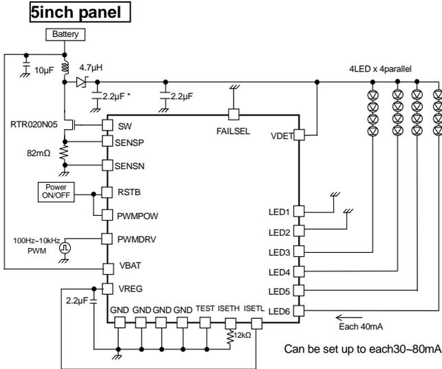
Figure 58. 4 series x 4 parallel, LED current 40mA setting
