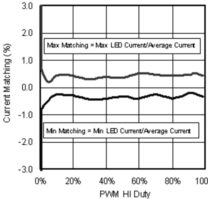
Figure 17. LED current matching - PWMDRV-HI Duty PWM = 200Hz
