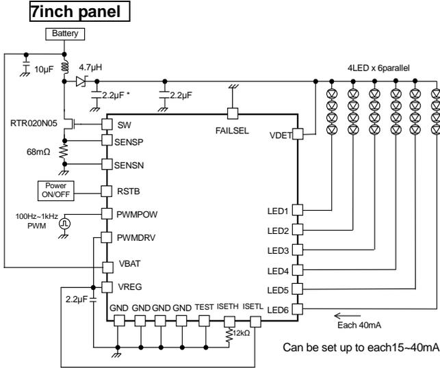
Figure 54. 4 series x 6 parallel, LED current 40mA setting Power control PWM application
