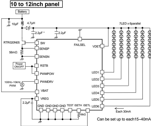
Figure 50. 7 seriesx6 parallel, LED current 30mA setting Current driver PWM application
