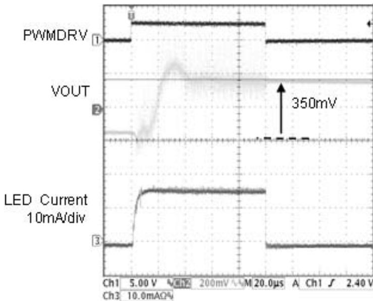
Figure 19. VOUT response Driver Control PWM (PWMDRV)
