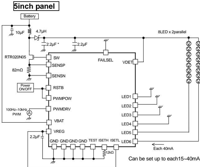
Figure 56. 8 series x 2 parallel, LED current 40mA setting Current driver PWM application
