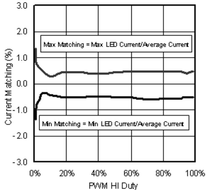
Figure 20. LED current matching - PWMPow-HI Duty PWM = 200Hz
