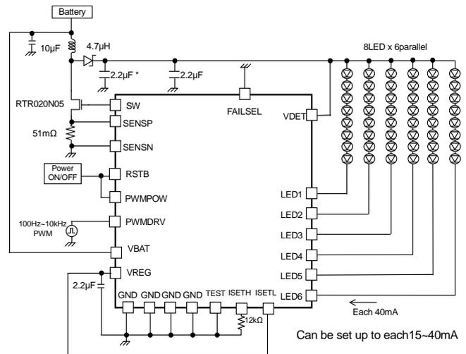
Figure 49. 8 seriesx6 parallel, LED current 40mA setting Current driver PWM application
