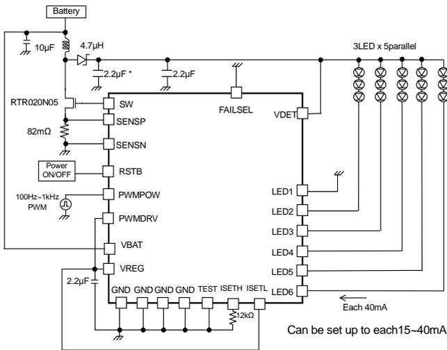
Figure 60. 3 series x 5 parallel, LED current 40mA setting
