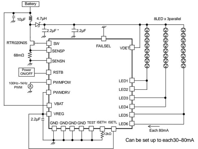
Figure 55. 8 series x 3 parallel, LED current 80mA setting Power control PWM application
