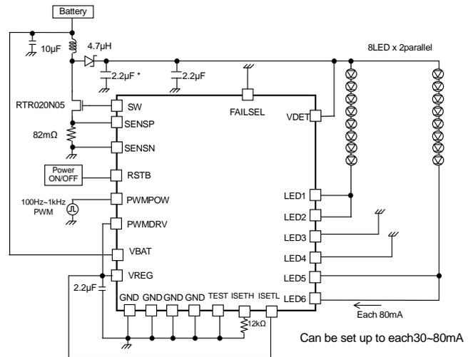
Figure 57. 8 series x 2 parallel, LED current 80mA setting Power control PWM application
