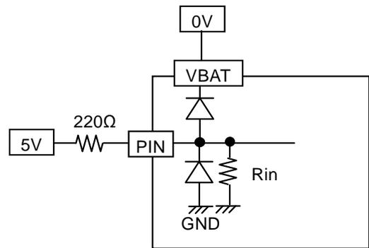
Figure 34. Voltage with a control sign higher than VBAT
