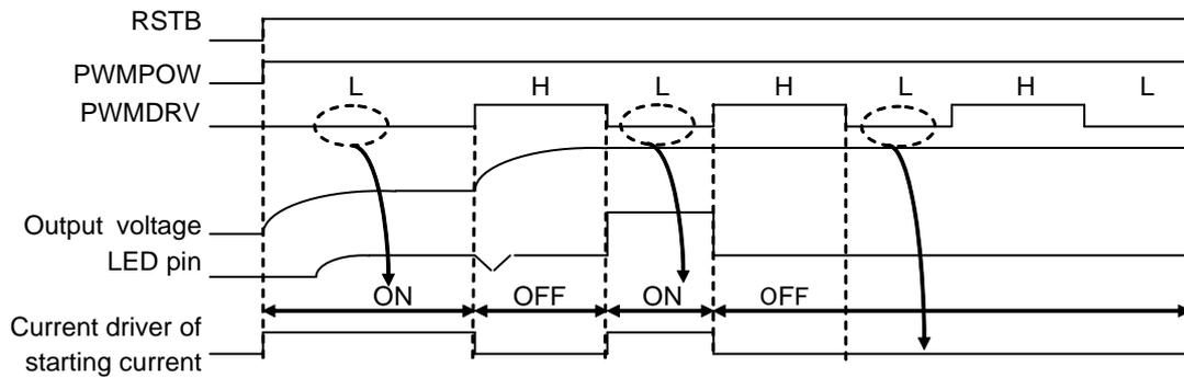
Figure 38. Off timing of starting current at PWMDRV=L
