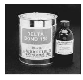
DeltaBond™ 154 is a medium viscosity, aluminum-filled resin with the best thermal conductivity of this series. It is, however, neither a good electrical insulator nor conductor. Its principal application is that of a good thermal mechanical adhesive for applications such as bonding fins to base plates or structural mounting blocks or brackets to heat sinks. Order one bottle of hardener A4 or B4 per one quart of DeltaBond™ 154 separately. Shelf life: 3 years.
