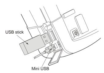
Figure 35. Test Tool USB Connections
