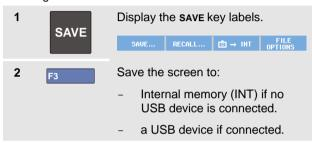
The file is saved using a fixed name (IMAGE) and a serial number, for example IMAGE004.bmp.
