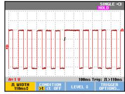
Figure 34. Triggering on Missing Pulses
