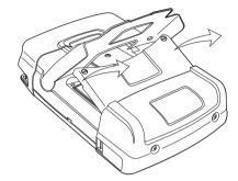
Figure 48. Removing the Battery Cover
