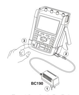
Figure 2. Powering the Test Tool
