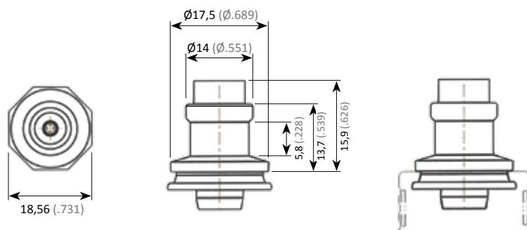
**STRAIGHT BACKSHELL FOR SIZE 8 SOCKET MODULES**
