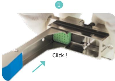
The module extraction is carried out using a blue tool P/N **006101 000 00**, except RJ45 and EN4830 optic modules using a green tool P/N **006101 008 00** (page 95).
