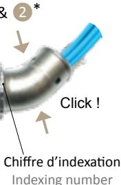
Assembly both half-chimneys around the cable harness.
