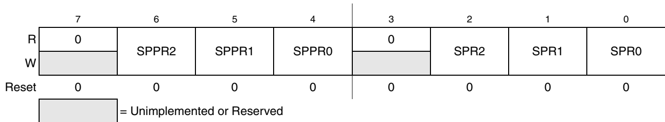
Figure 15-7. SPI Baud Rate Register (SPIxBR)
