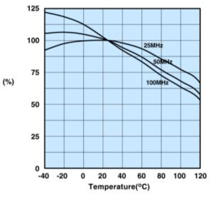
Measured on a 2643000301 using the HP4291A.
