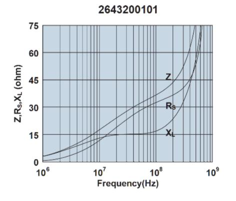
Impedance, reactance, and resistance vs. frequency.
