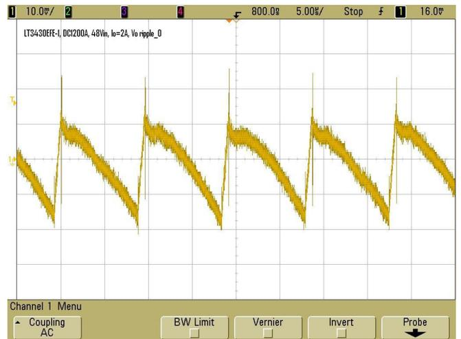
Figure 5. Typical VOUT ripple 48VIN 2A load
