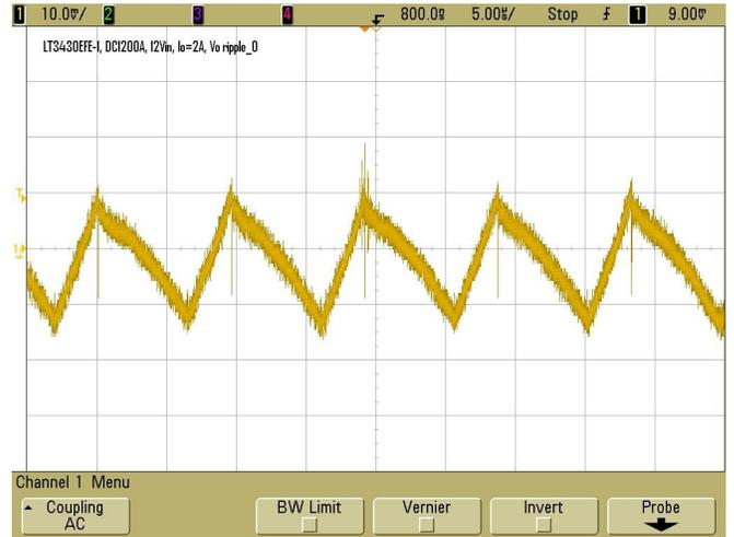
Figure 4. Typical VOUT ripple 12VIN 2A load
